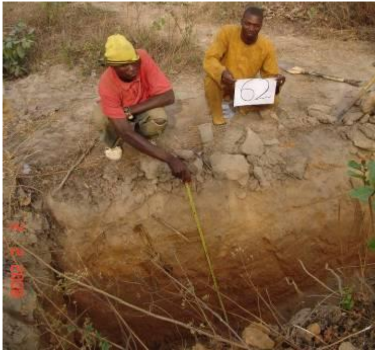
Picture No. 33 Exposed profile of alluvium secondary river soil in a typical digging point
