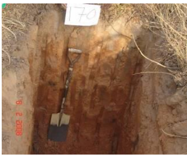
Picture No. 29 Exposed profile of Yellow – brown soil in a typical digging point
